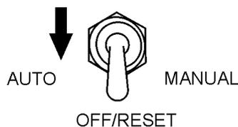
**Figure 56. MPEC Control Switch (Off/Reset)**
