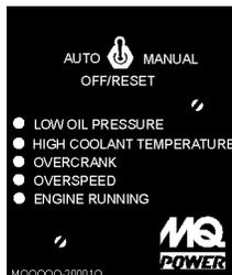
and all major faults will shutdown the generator. During cranking cycle, the ECU will attempt to crank the engine for 10 seconds before disengaging.
