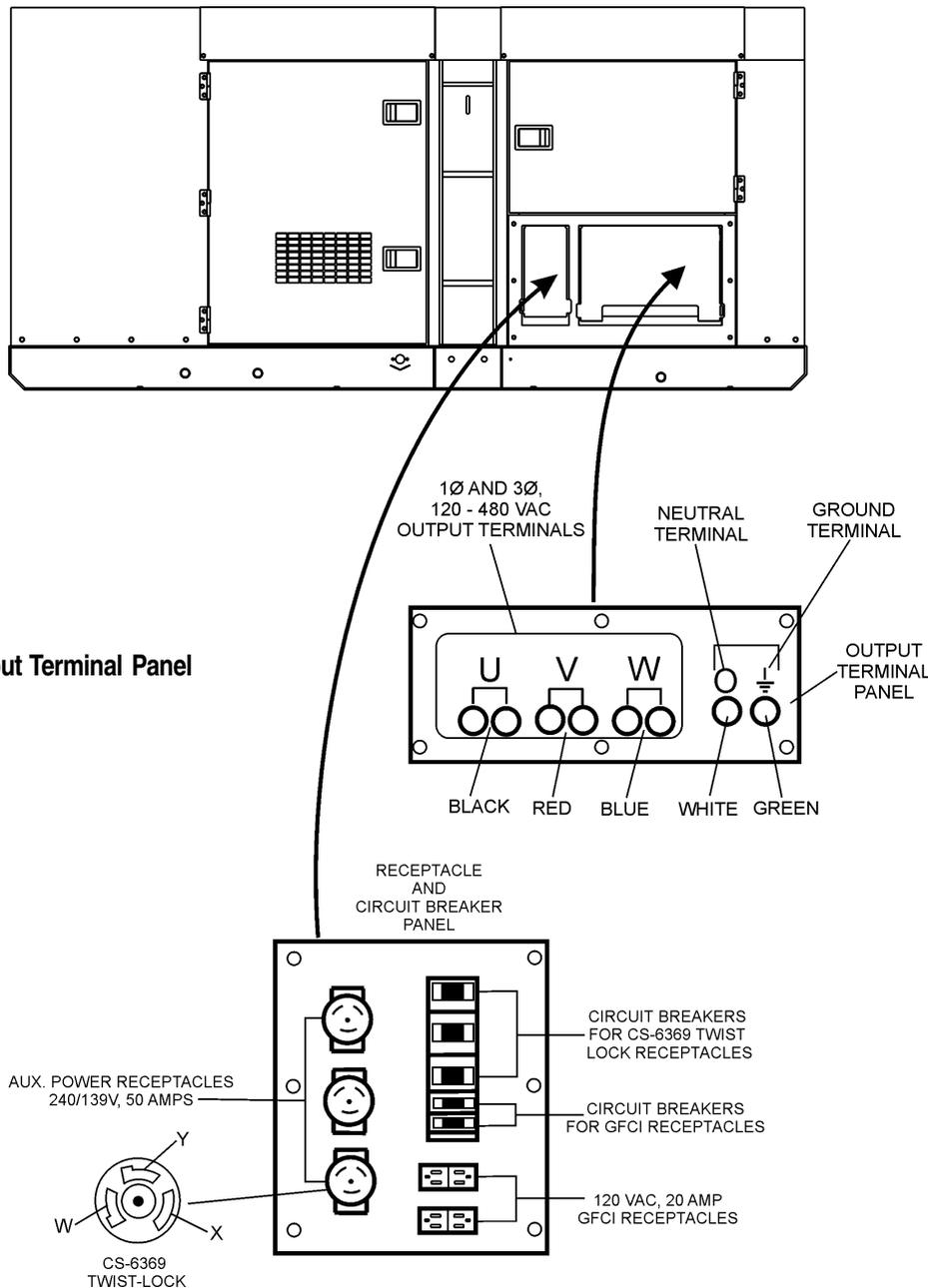
Figure 8. Output Terminal Panel
