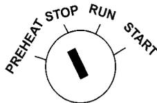
**Figure 69. Ignition Key Switch (STOP position)**
