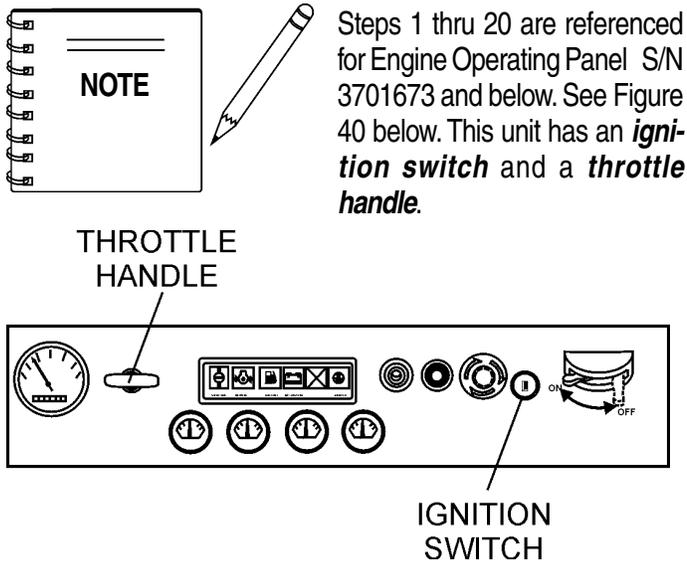
Figure 40. Engine Operating Panel S/N 3701673 and Below
