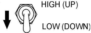
**Figure 71. Engine Speed Switch (High)**
