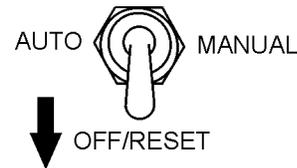
**Figure 72. Auto-Manual Off/Reset Switch**
