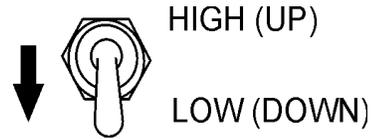
Figure 60. Engine Speed Switch (Low)
