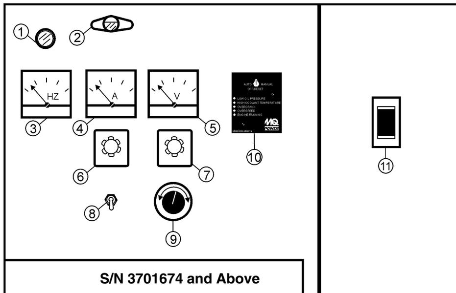
Figure 6. Generator Control Panel
