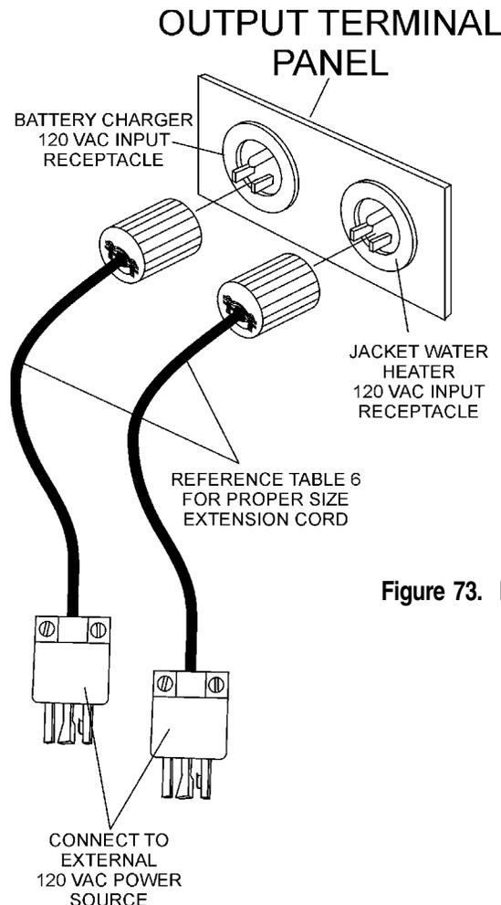
Figure 73. Battery Charger/Jacket Water Heater Power Connections
