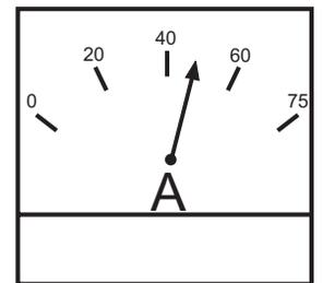
Figure 19. AC Ammeter (Amp reading on U lug)
