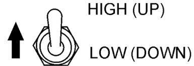
Figure 62. Engine Speed Switch (High)
