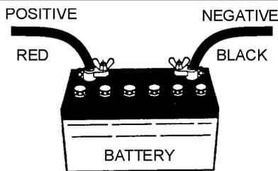
**Figure 39. Battery Connections**
