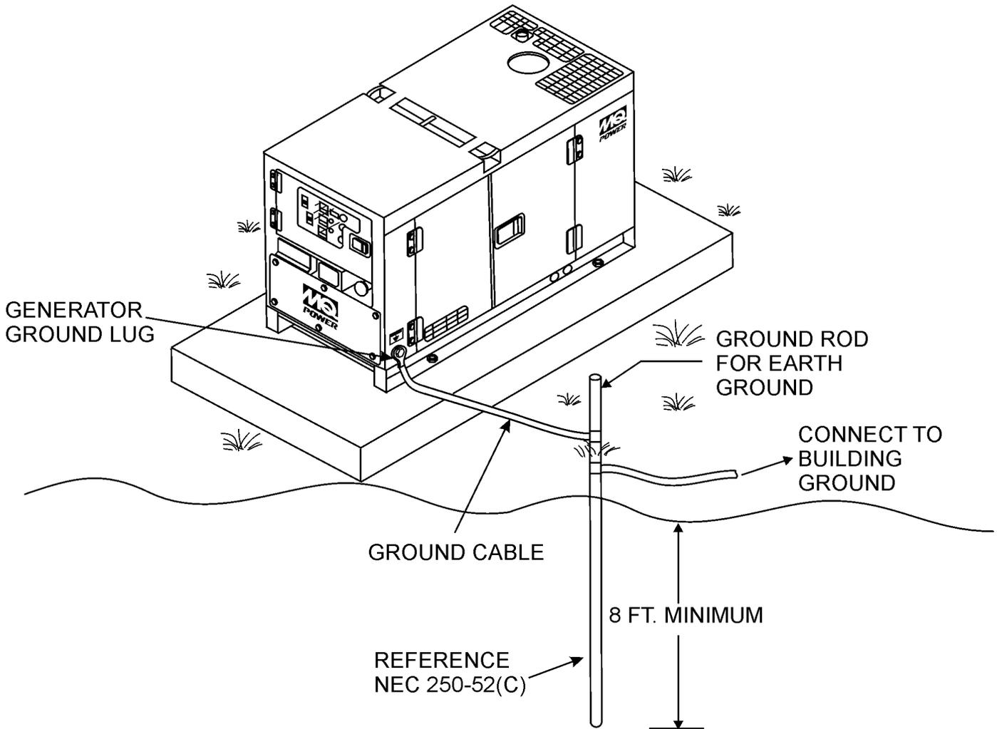
Figure 4. Typical Generator Grounding Application
