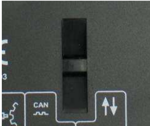
Cable Tie Fixing Point
