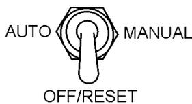
Figure 52. Off/Manual Auto Switch (OFF)
