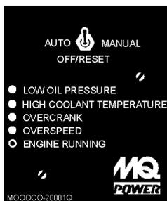
**Figure 50. Engine Controller Status LED**
