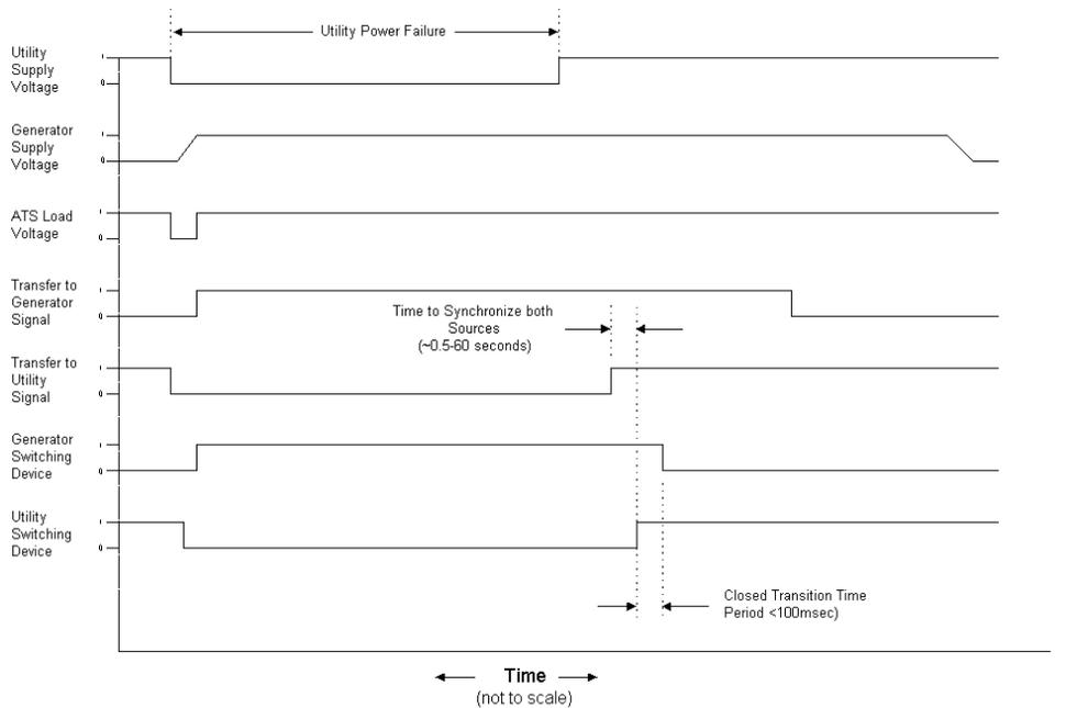
The following operating sequences and time delays are associated with closed transition type transfer switches which momentarily parallel two sources of supply for less than 100 milliseconds. For closed transition type transfer switches, which utilize extended parallel operation for soft-loading operating sequences, refer to separate instruction manual.
