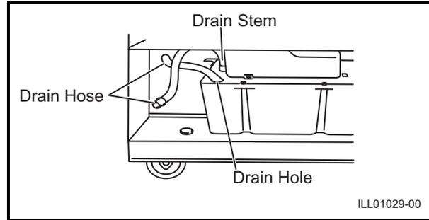
**Note:** The pump's maximum lift is 17 feet (5.2 m) at 230VAC (13 feet (4 m) at 208VAC). Please check the drainage performance after installation. It is important that the drainage line from the pump is free of kinks and is not pinched. Power fluctuation or low voltage could result in incorrect drainage.
