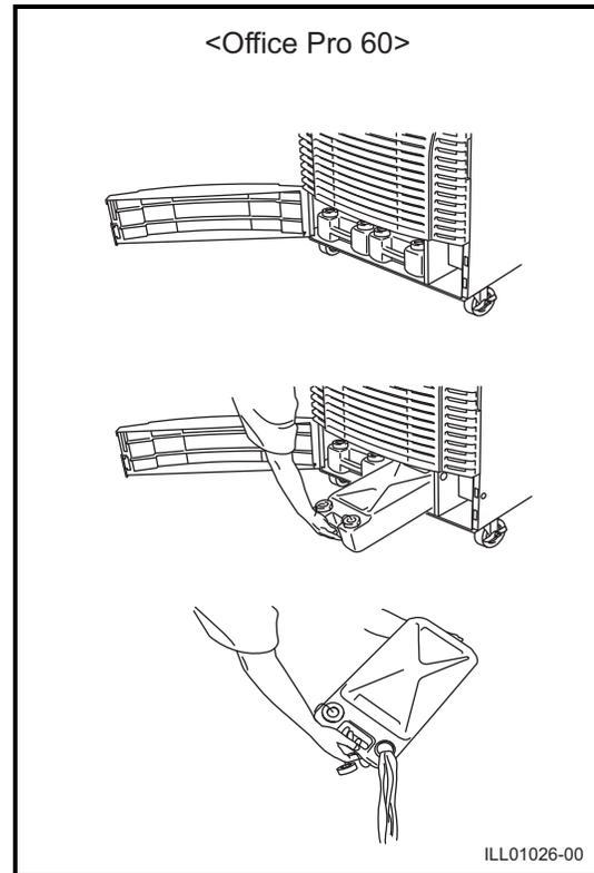
1. Open the front panel of Office Pro 36 or drain tank door of Office Pro 60.
