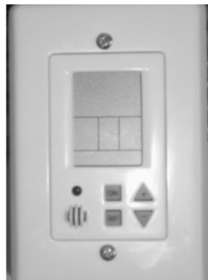
Figure 9 – Remote Thermostat Control
